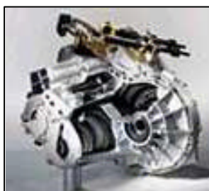
Figure C6.1 - Example of five speed manual transverse installed transmission
