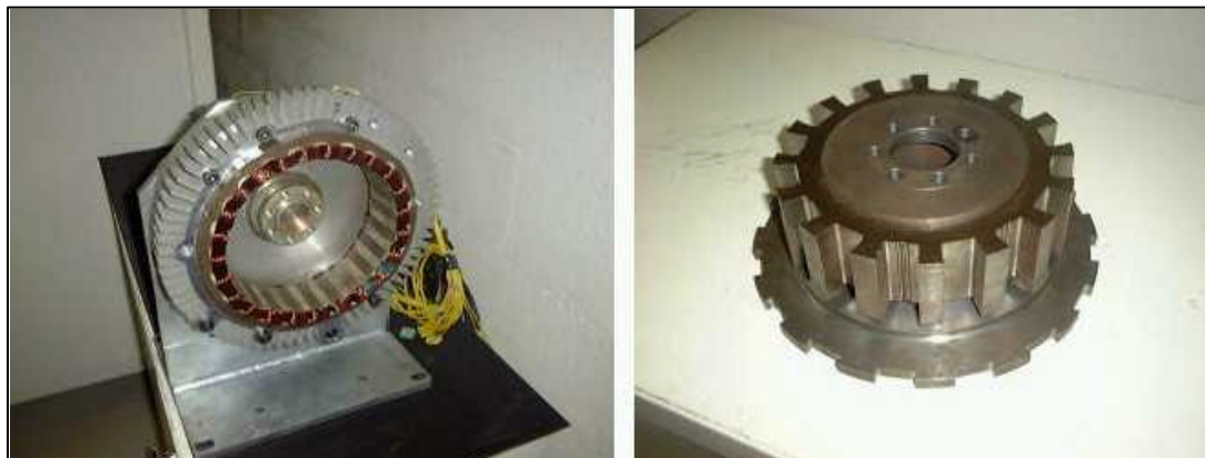
Figure C2.3 - Crankshaft mounted Switched Reluctance Motor / Generator
